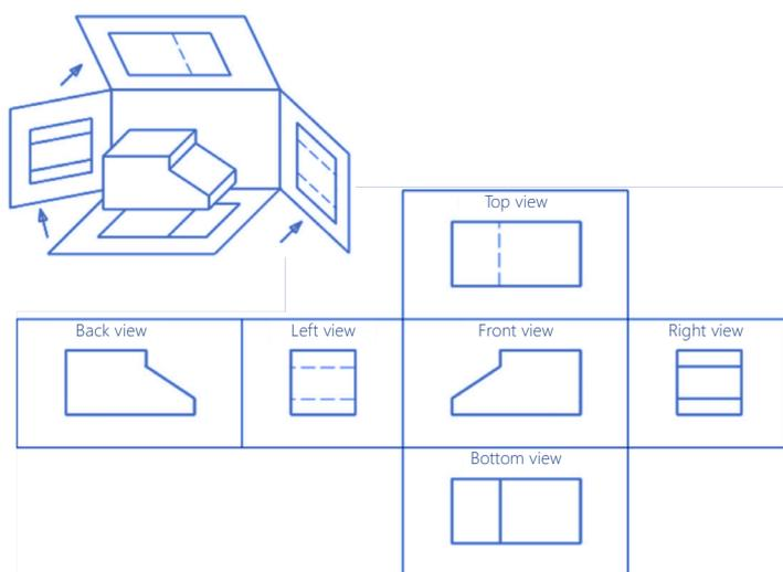
**You can start by defining what the left, right, top, and bottom views are, by using the "projection cube" principle:**
