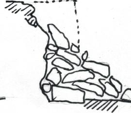
4) WALL IS REBUILT WITH EXTRA DEPTH, STONES LEAN INWARDS
