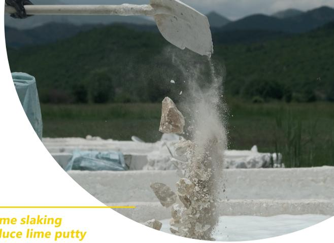
**Quicklime slaking to produce lime putty**
