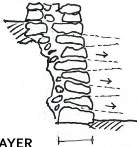
2) SOIL PRESSURE CAUSES WALL TO BULGE
