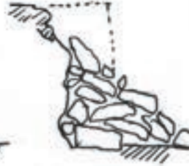
3) WITH RAINFALL, THE WALL COLLAPSES
